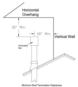
Figure 15 - Termination Cap clearances
