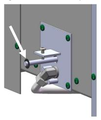
Figure 40 - Air Shutter Closed
