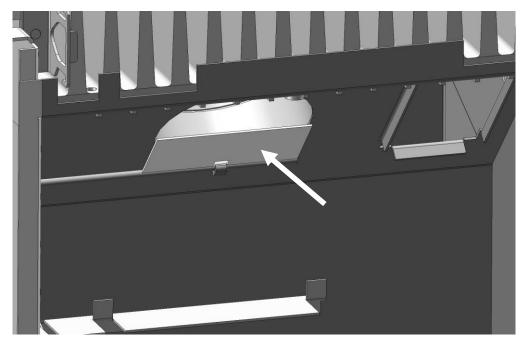
Figure 19 - Restrictor Fully Closed Detail (baffle removed for clarity)
