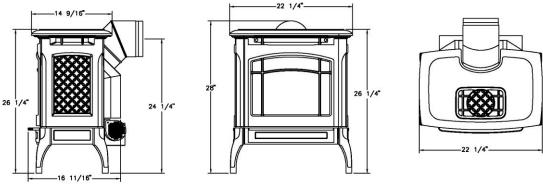
Shown with optional 45° Elbow. Blower is standard and is factory installed.
