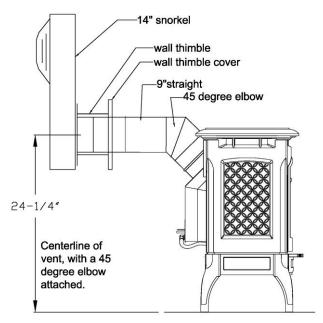
Figure 17 - Components for a Typical Snorkel Installation
