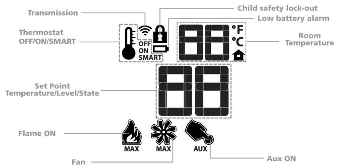
Figure 5 - GTMF Remote Transmitter Display Data
