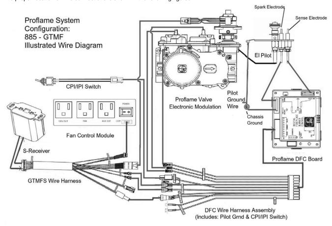
Figure 22 - Stowe DX Wiring Diagram
