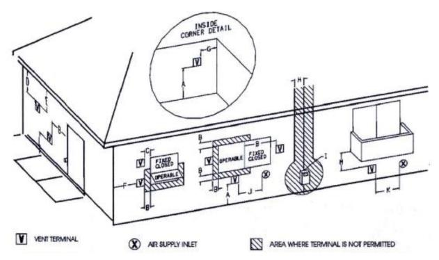
Figure 16 - Acceptable Direct Vent Terminal Vent Cap Locations
