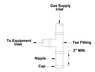
Figure 25 - Sediment Trap (Typical)
